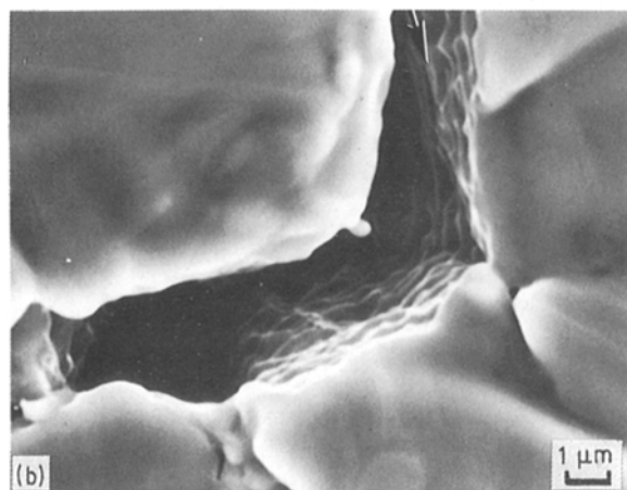
Figure 6 Morphological features of as-welded Sandvik HT-9 containing 1 a.p.p.m. He. (a) Intergranular fracture along prior-austenite grain boundaries, (b) grain-boundary facets decorated with a uniform distribution of dimples.
